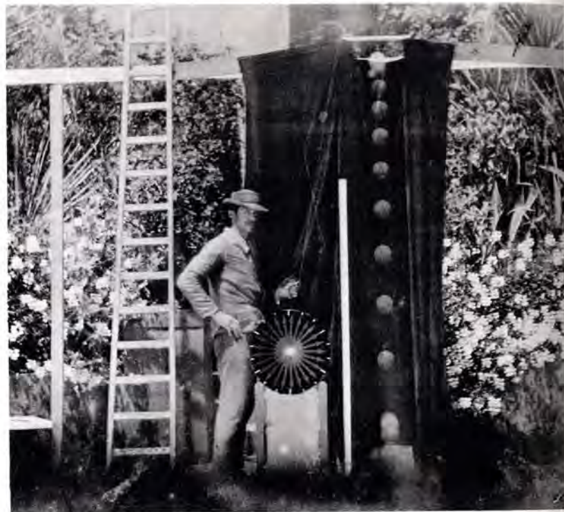
ETIENNE JULES MAREY. Serial photograph showing acceleration of falling ball. c. 1887. Courtesy of André Jammes
